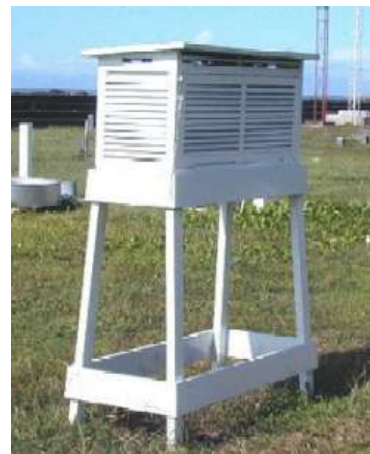
7. A Stevenson screen. This houses maximum and minimum and dry and wet bulb thermometers. Source: Samoa Meteorology Division.
