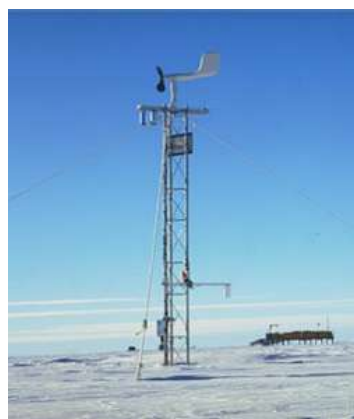
8. An automatic weather station. This station is equipped with a solar panel and records temperature, water vapour, wind direction, wind speed and air pressure. The data are transferred by satellite. Other measurement equipment at the station provides local weather information for local aviation. Source: AWI.
